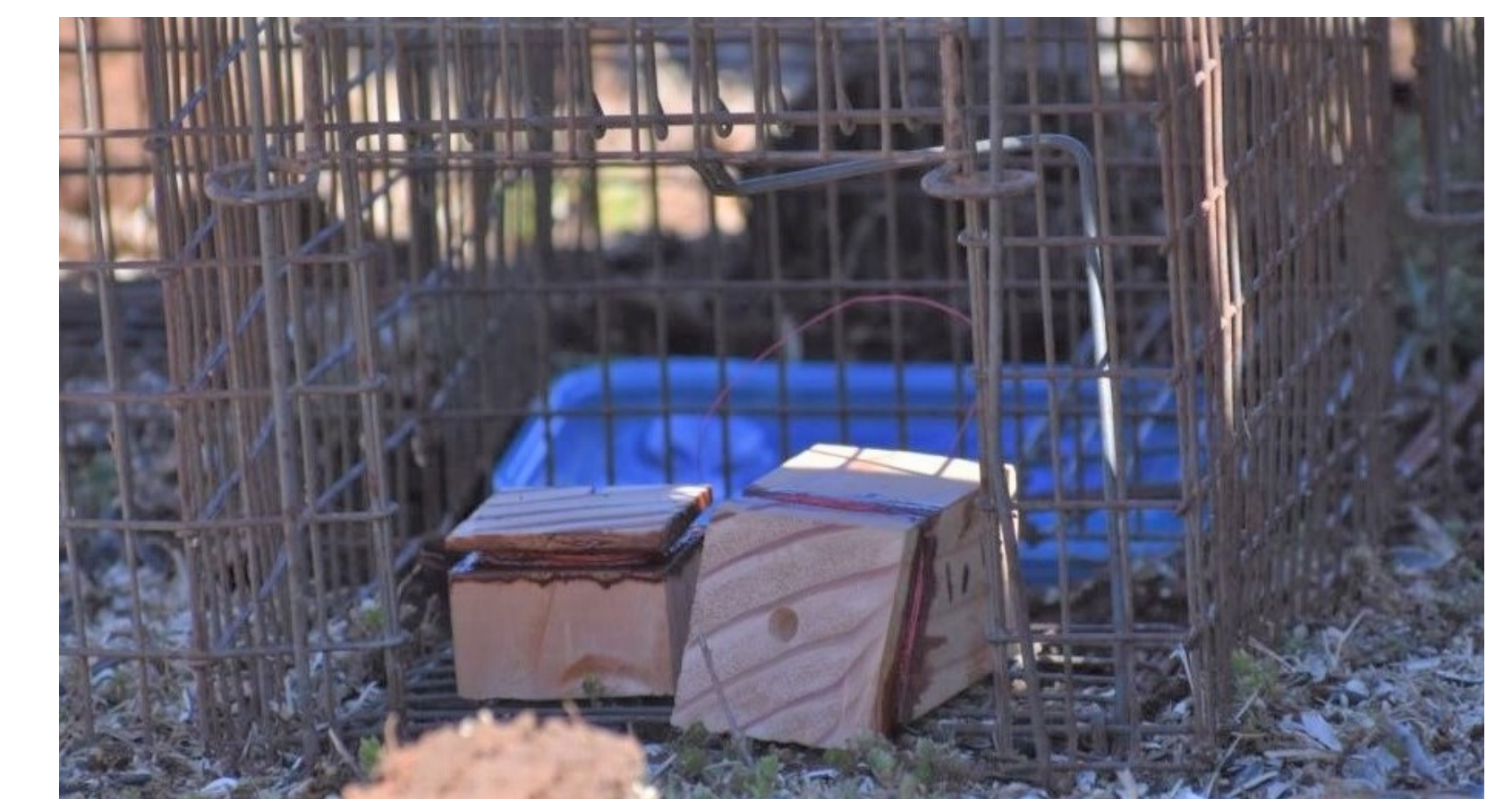
Figure 6: Initial RFID Set-up (removed because of durability issues)
